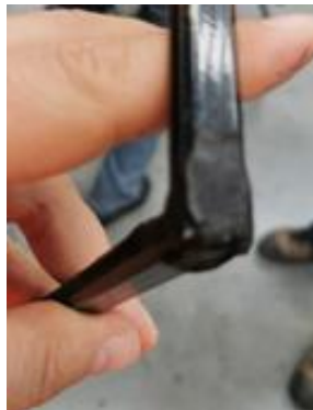
Welded corner key secured with butyl
