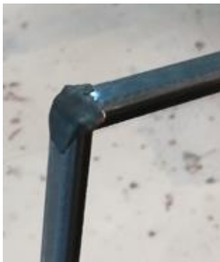
Bended corner secured with butyl
